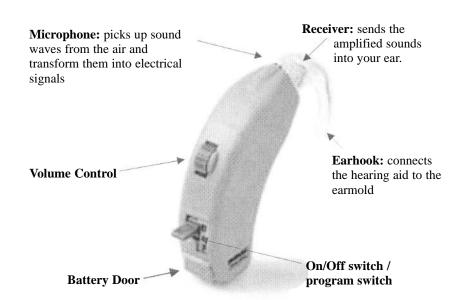
Hearing aids are an electronic device that amplifies sound at different levels for different pitches. A hearing aid consists of a microphone, amplifier and receiver.
